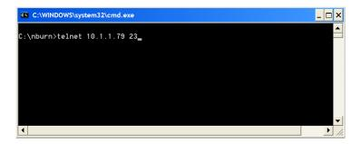
**6.** At this point, anything you type in the Telnet window should appear in the serial terminal window and vice versa.
