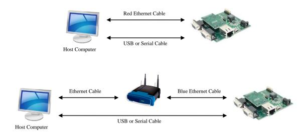
The objective of this example is to use a single host computer running Telnet and a serial terminal program to send data in either direction. When you type text in the Telnet window, it should appear in the serial terminal window and vice versa.
