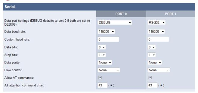
The SBL2e provides two TTL level UARTs: Port 0 and 1. The "RS-232", "RS-485 Half Duplex" (Port 0 only), and "RS-485 Full Duplex" (Port 0 only) data port settings will enable the TTL level signals. You will need to add external level shifters if RS-232/RS-485 electrical signals are needed instead of 0-3.3V DC TTL.
