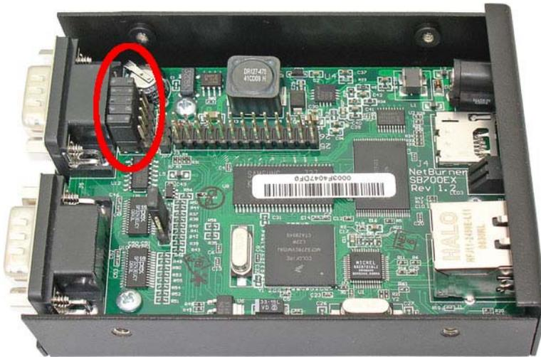
The jumper locations are shown below. The two red jumpers are used for half-duplex, both the red and blue are required for full duplex.
