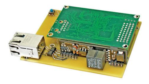
PoE adapter board with SBL2e installed.
