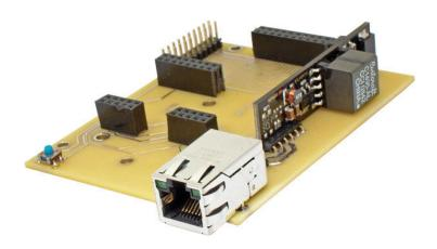
PoE adapter board with SB70LC Development Board connected to provide serial port level shifters and DB9 connectors
