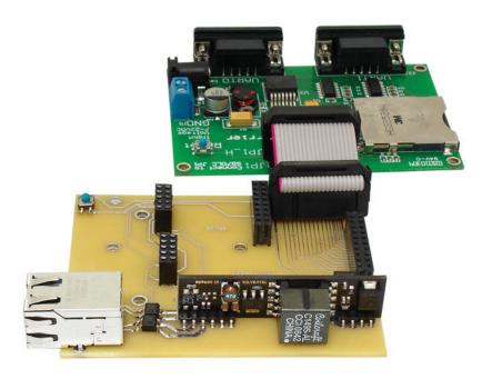
PoE adapter board with SB70LC installed.
