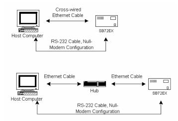
The objective of this example is to use a single host computer running telnet and a serial terminal program to send data in either direction. Therefore, if you type text in the telnet window, it should appear in the serial terminal window and visa versa. For a serial terminal, you can use MTTTY (which is included in your NetBurner PK70 CD-ROM) or HyperTerminal.
