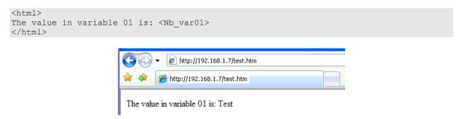
Save the file as **test.htm**. Open an FTP connection as outlined previously and copy the file to the PINK Module. Browsing to **XXX.XXX.XXX/test.htm** (where **XXX.XXX.XXX.XXX** is the IP Address of the PINK Module) displays the web page you just created. Using the Modify Variables web page (in another window) you can change the value of variable 01 then refresh the original test browser page to see the results change. If you haven't set the variable it will most likely contain **NA**.
