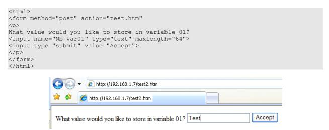
Save the file as test2.htm and copy the file to the PINK Module using the previously discussed FTP methods. Browsing to **XXX.XXX.XXX.XXX/test2.htm** (where **XXX.XXX.XXX.XXX** is the IP Address of the PINK Module) opens a form page that can be used to change the value in variable 01. Once the 'Accept' button is clicked the original **test.htm** page will be loaded to display the new value.
