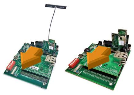
**Note**: Plug in WiFi Adapter Board with component side towards the Ethernet Core Module!
