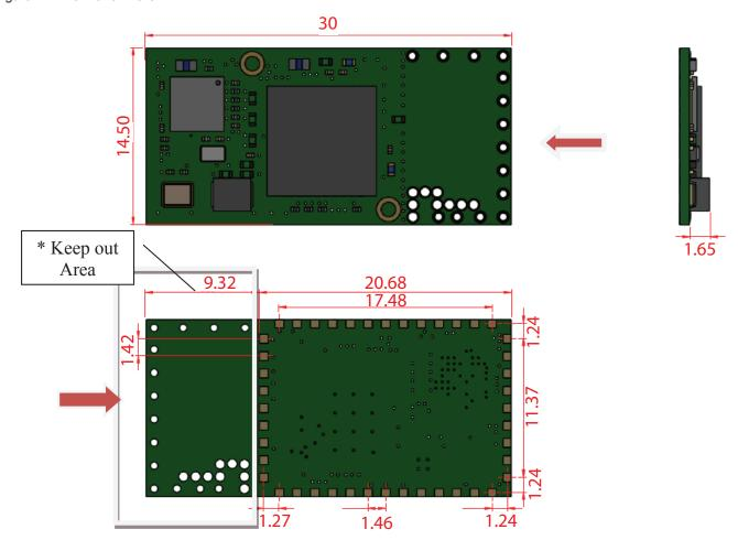
"Keep out" area should ideally have the antenna hanging off the side of the PCB for best performance. If you do not hang the antenna off the PCB, ensure no ground planes or traces are placed under the antenna (keep out area). Surrounding metal will affect the antenna performance. \* External Antenna does not require "keep out" area
