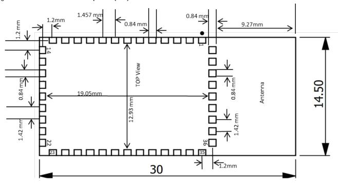
Figure 3: PCB Recommended Footprint - Top View (mm)
