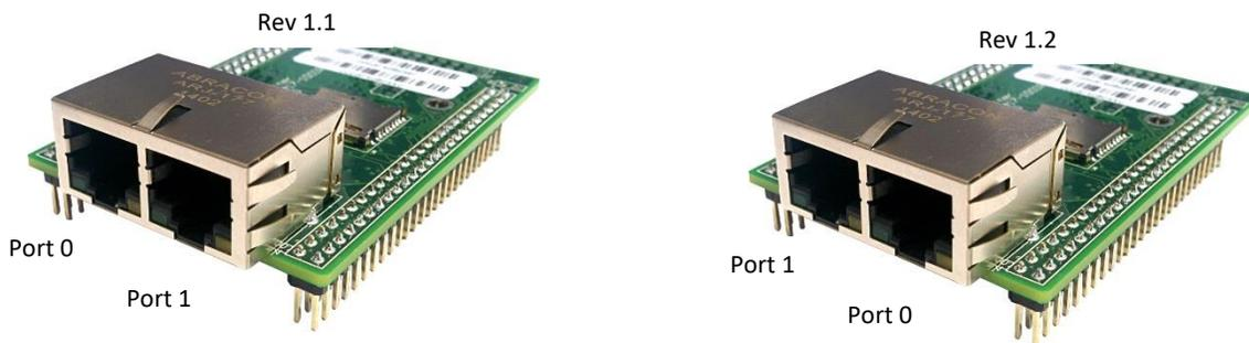
Note: above images show the -100 version with the Ethernet jacks installed. This change effects the -200 version in the same manor.
