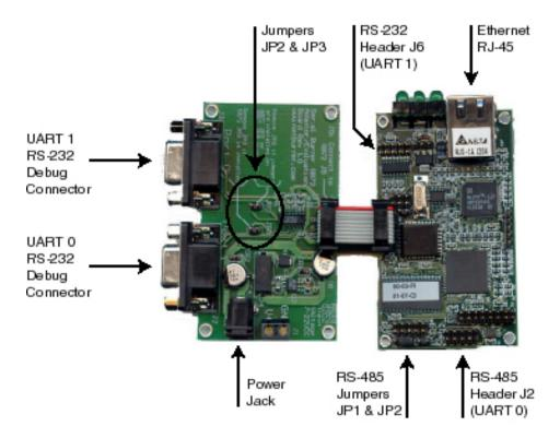
Figure 2: SB72 w/ SB72 Adapter Board
