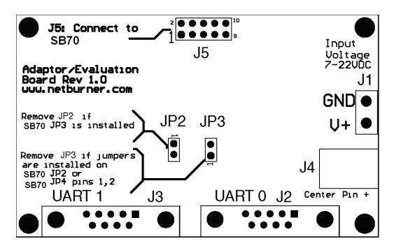
Figure 3: SB72 Adapter Board Connector Pinouts
