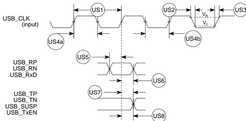
**Figure 23-22. USB Interface Timing****23.12 IEEE 1149.1 (JTAG) AC Timing Specifications**
