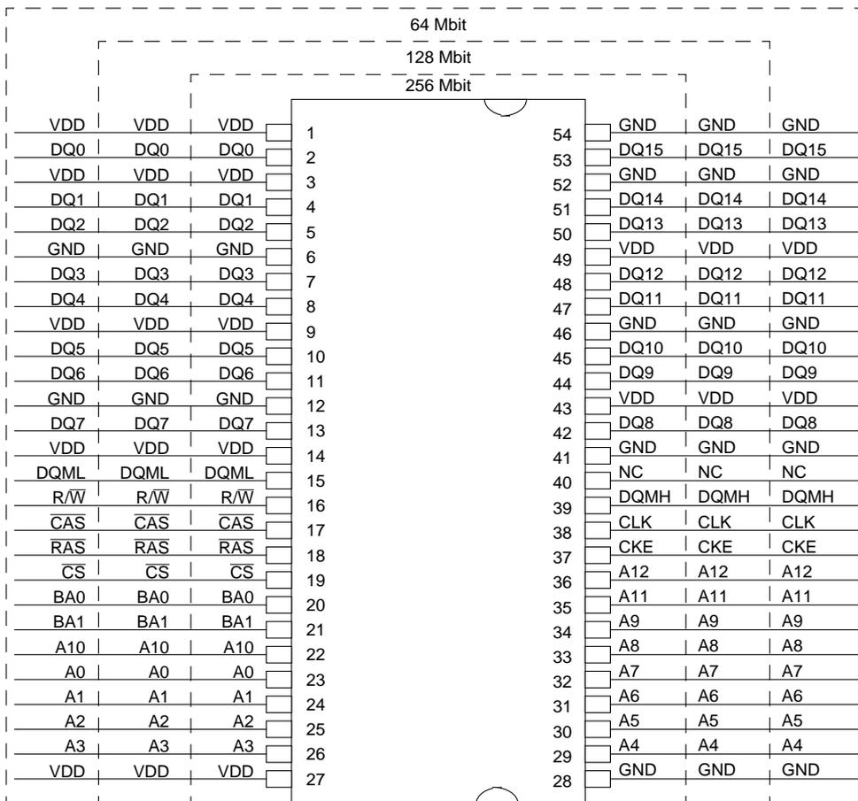
**Figure 9-2. 54-Pin TSOP SDRAM Pin Definition**
