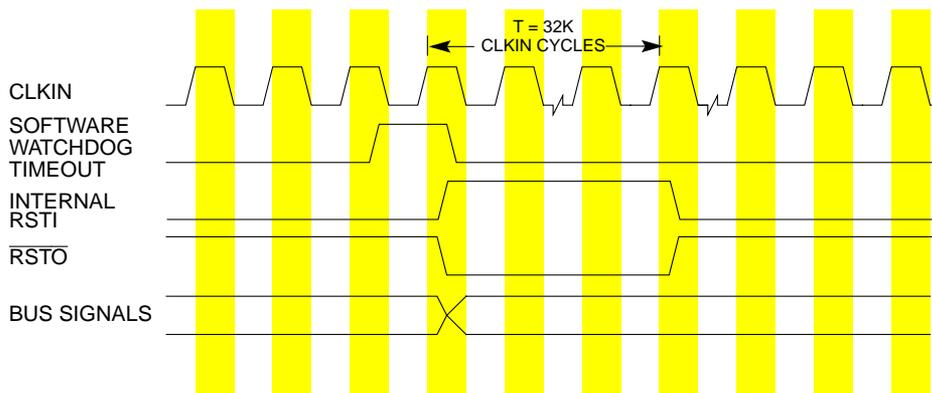
Figure 20-23. Software Watchdog Timer Reset Timing
