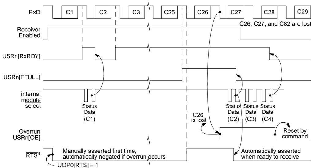
**Figure 16-26. Receiver Timing**
