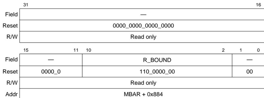
**Figure 11-12. FIFO Receive Bound Register (FRBR)**
