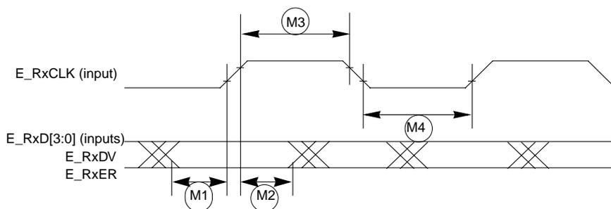
**Figure 23-11. MII Receive Signal Timing Diagram**
