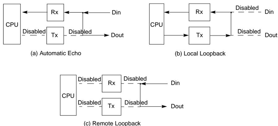
Figure 13-9. GCI/IDL Loopback Mode
