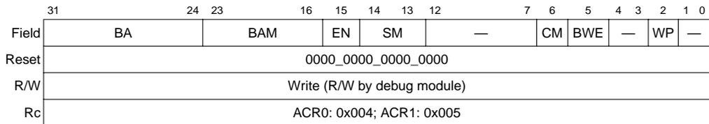
**Figure 4-5. Access Control Register Format (ACR<sub>n</sub>)**
