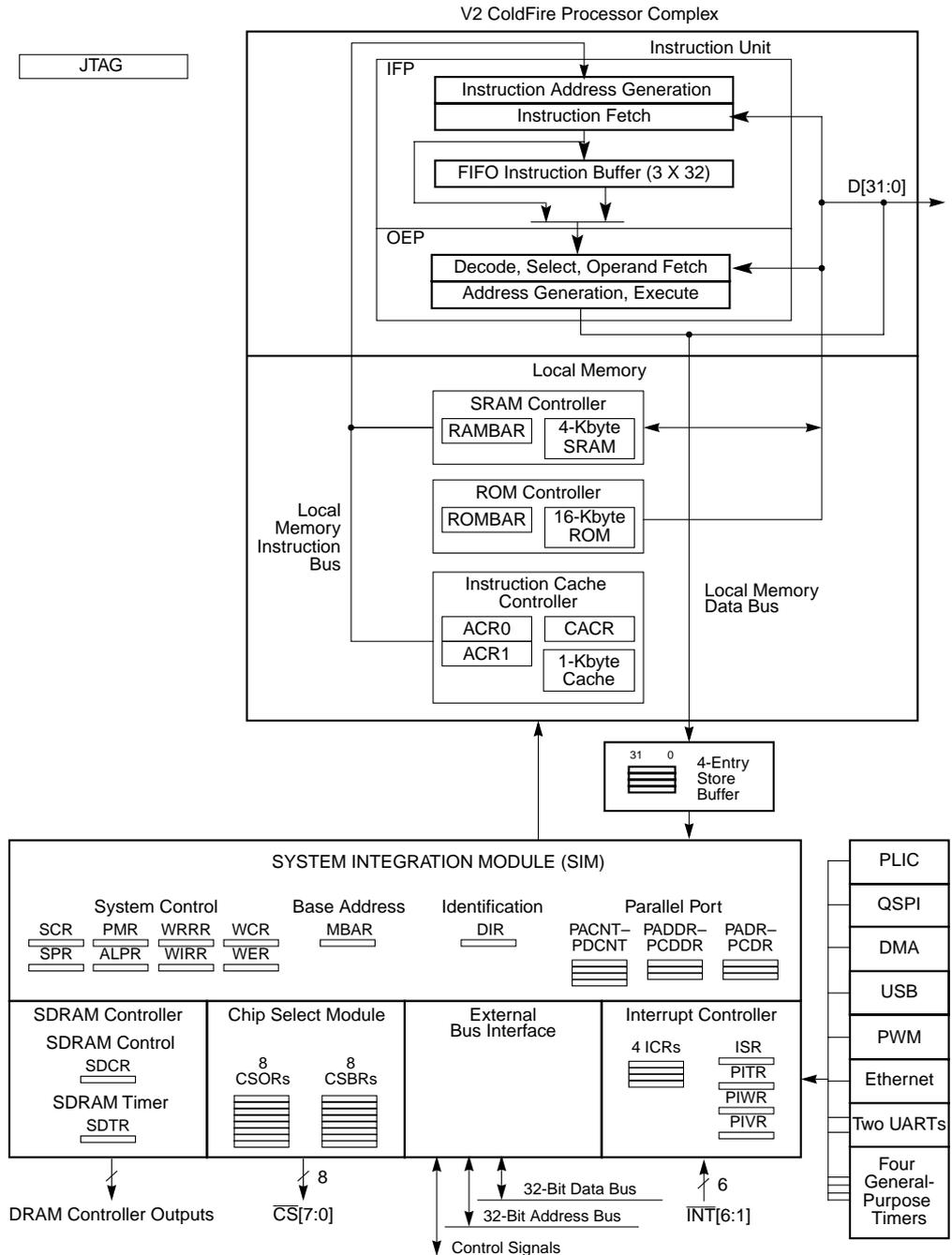
Figure 1-1. MCF5272 Block Diagram
