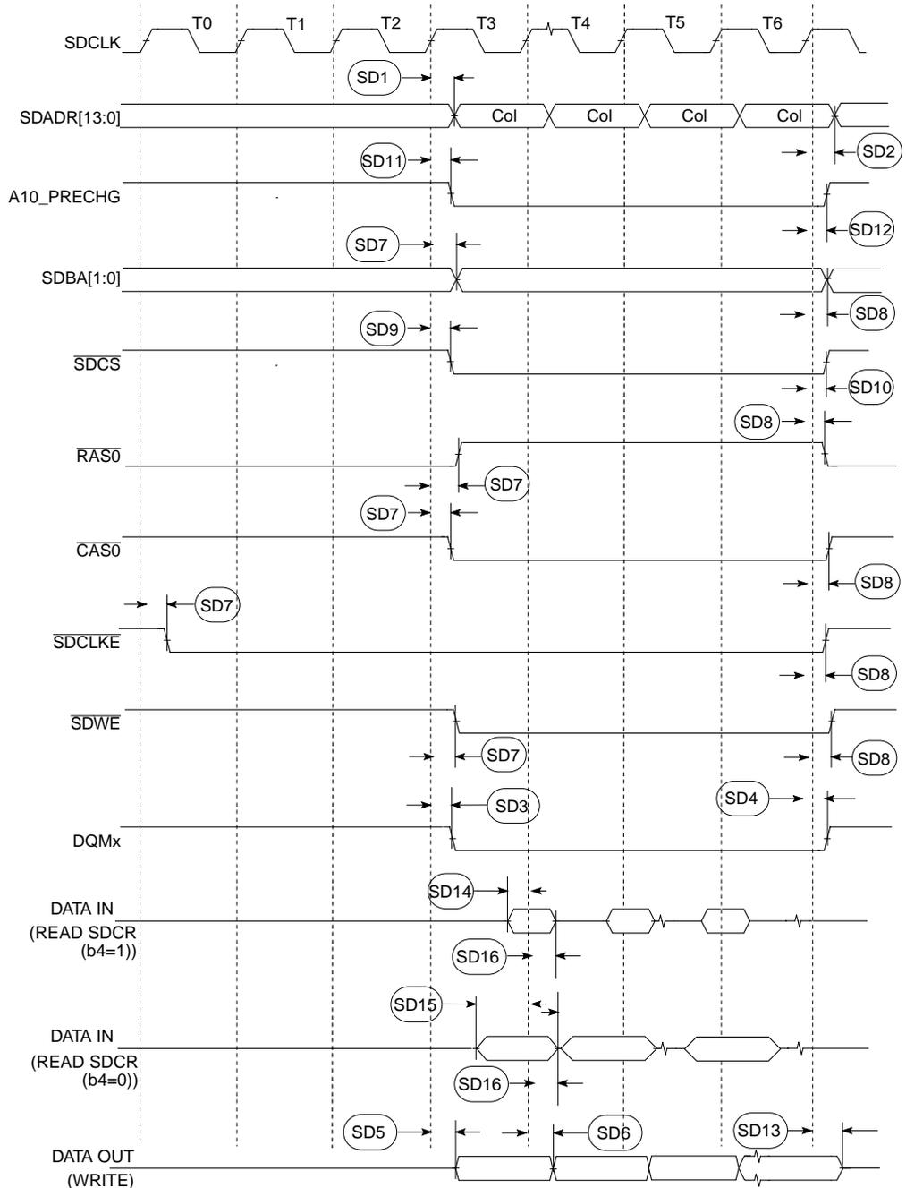
Figure 23-9. SDRAM Signal Timing
