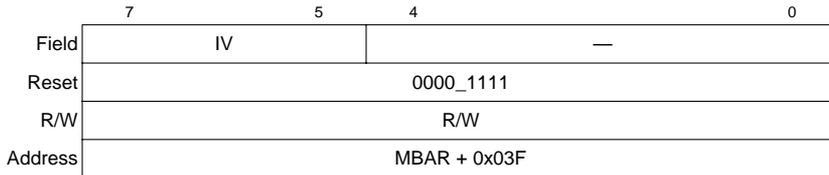
**Figure 7-9. Programmable Interrupt Vector Register (PIVR)**
