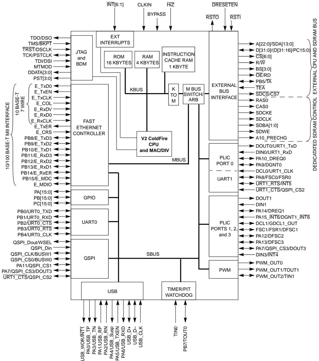
NOTE: GPIO pins shown above are multiplexed with most other signals.
