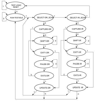
Figure 21-2. TAP Controller State Machine
