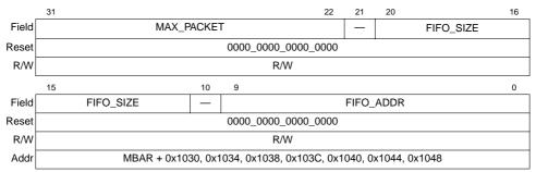
Figure 12-15. USB Endpoint 1-7 Configuration Register
