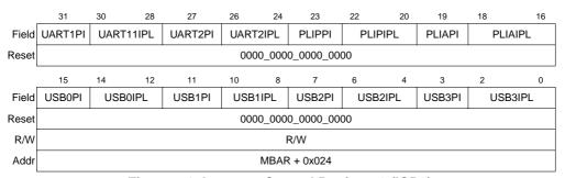
Figure 7-3. Interrupt Control Register 2 (ICR2)
