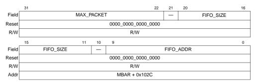
Figure 12-14. USB Endpoint 0 OUT Configuration Register
