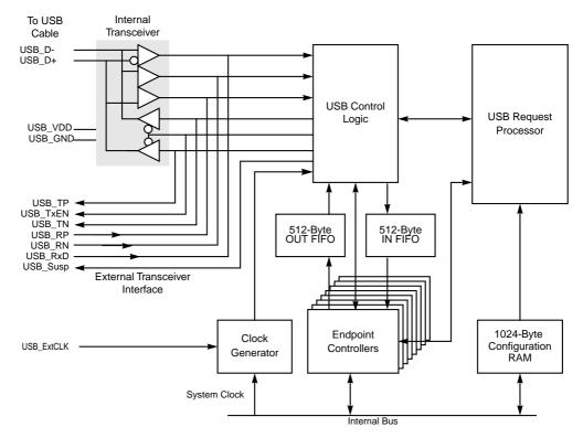
Figure 12-2. USB Module Block Diagram
