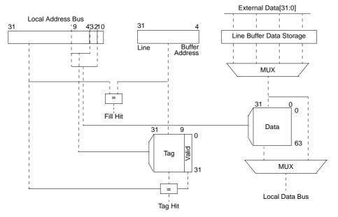
Figure 4-3. Instruction Cache Block Diagram
