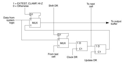
Figure 21-3. Output Cell (O.Cell) (BC-1)
