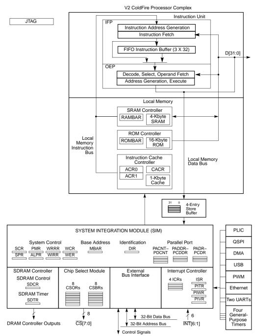
Figure 1-1. MCF5272 Block Diagram
