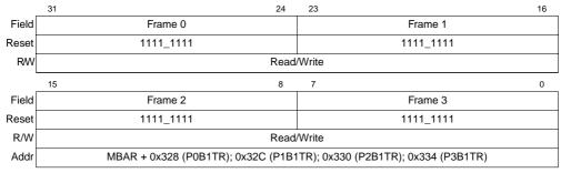
Figure 13-16. B1 Transmit Data Registers P0B1TR-P3B1TR
