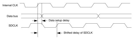
Figure 9-6. Timing Refinement with Inverted SDCLK
