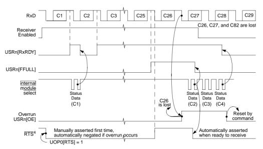
Figure 16-26. Receiver Timing
