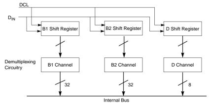
Figure 13-2. GCI/IDL Receive Data Flow
