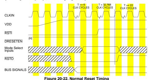
The levels of the mode select inputs, QSPI\_Dout/WSEL, QSPI\_CLK/BUSW1, QSPI\_CS0/BUSW0, and  $\overline{\text{HiZ}}$  are sampled when  $\overline{\text{RSTO}}$  negates and select the port size of  $\overline{\text{CSO}}$  and the physical data bus width after a master reset occurs.  $\overline{\text{RSTO}}$  is asserted as long
