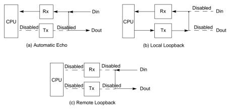
Figure 13-9. GCI/IDL Loopback Mode
