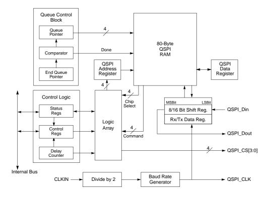
Figure 14-1. QSPI Block Diagram
