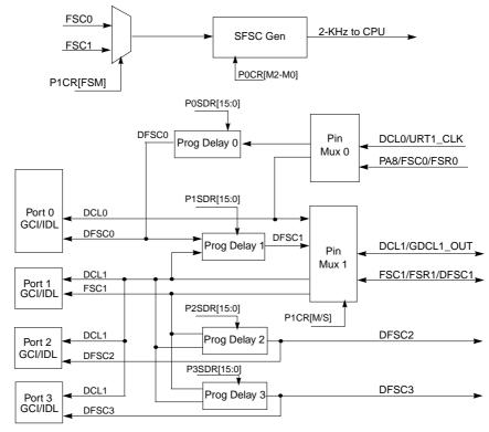
Figure 13-11. PLIC Internal Timing Signal Routing
