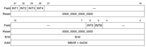
Figure 7-7. Programmable Interrupt Transition Register (PITR)
