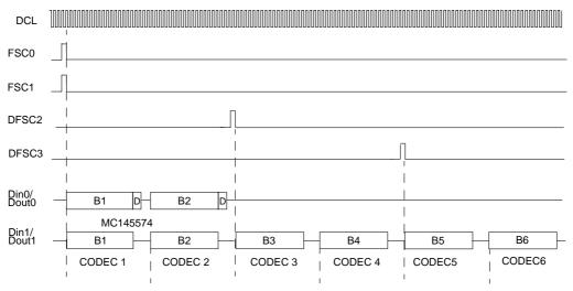
Figure 13-38. Standard IDL2 10-Bit Mode
