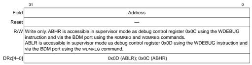
Figure 5-6. Address Breakpoint Registers (ABLR, ABHR)
