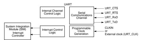
Figure 16-1. Simplified Block Diagram
