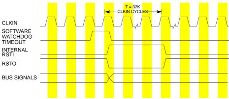
Figure 20-23. Software Watchdog Timer Reset Timing
