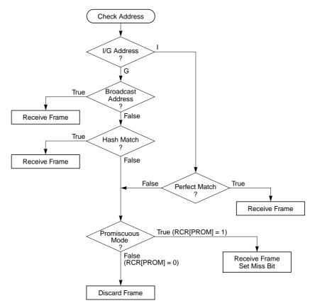
Figure 11-4. Ethernet Address Recognition Flowchart
