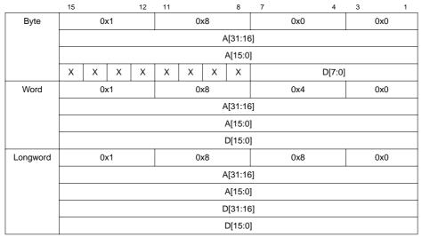
Figure 5-23. WRITE Command Format
