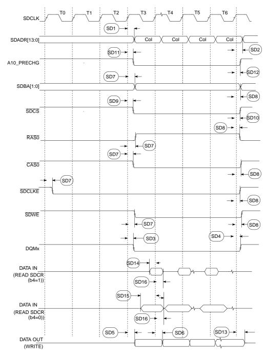
Figure 23-9. SDRAM Signal Timing
