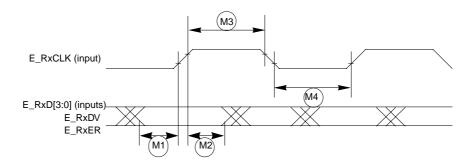
Figure 23-11. MII Receive Signal Timing Diagram
