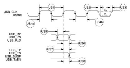
Figure 23-22. USB Interface Timing
