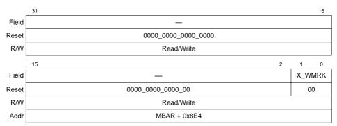
Figure 11-14. Transmit FIFO Watermark (TFWR)
