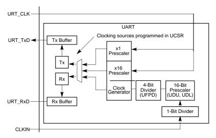
Figure 16-23. Clocking Source Diagram
