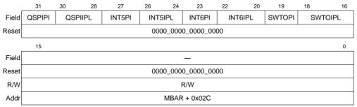
Figure 7-5. Interrupt Control Register 4(ICR4)
