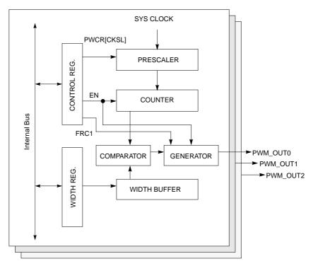
Figure 18-1. PWM Block Diagram (3 Identical Modules)
