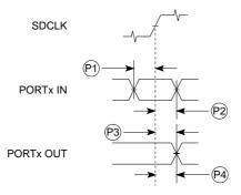
Figure 23-21. General-Purpose I/O Port Timing
