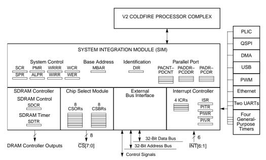
Figure 6-1. SIM Block Diagram
