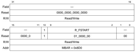
Figure 11-13. FIFO Receive Start Register (FRSR)
