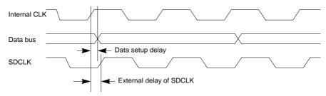
Figure 9-5. Example Setup Time Violation on SDRAM Data Input during Write
