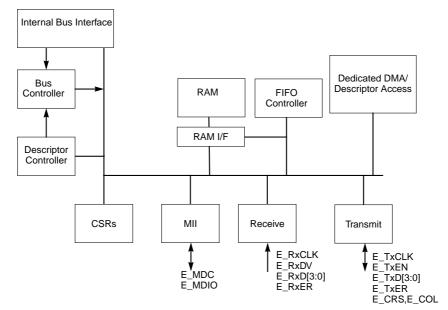
Figure 11-2. Fast Ethernet Module Block Diagram
