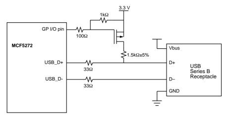
Figure 12-24. Recommended USB Line Interface
