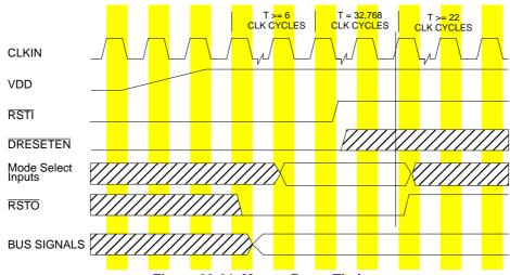
Figure 20-21. Master Reset Timing
