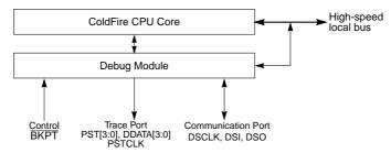
Figure 5-1. Processor/Debug Module Interface
