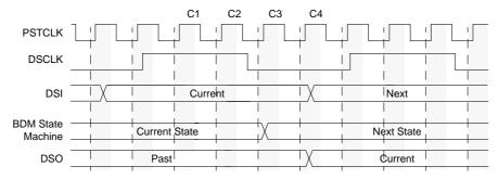
Figure 5-12. BDM Serial Interface Timing
