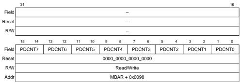
Figure 17-3. Port D Control Register (PDCNT)
