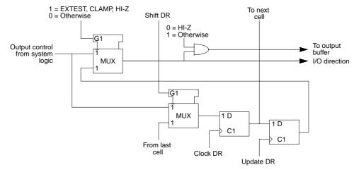
Figure 21-5. Output Control Cell (En.Cell) (BC-4)
