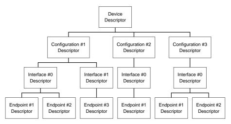
Figure 12-23. Example USB Configuration Descriptor Structure
