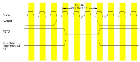
Figure 20-24. Soft Reset Timing
