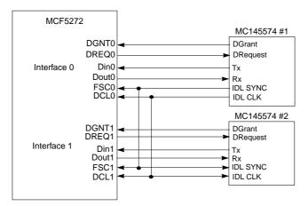
Figure 13-41. Two-Line Remote Access
