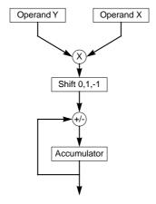
Figure 2-2. ColdFire Multiply-Accumulate Functionality Diagram
