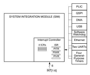
Figure 7-1. Interrupt Controller Block Diagram
