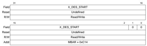
Figure 11-24. Pointer to Transmit Descriptor Ring (ETDSR)
