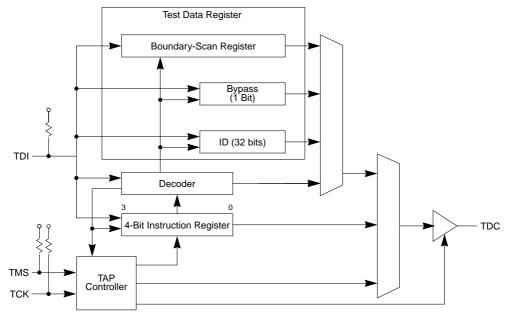
Figure 21-1. Test Access Port Block Diagram
