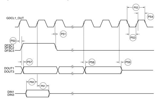
Figure 23-20. GCI Master Mode Timing
