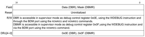
Figure 5-8. Data Breakpoint/Mask Registers (DBR and DBMR)
