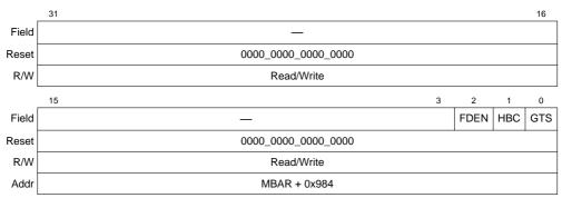
Figure 11-18. Transmit Control Register (TCR)
