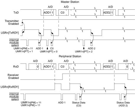
Figure 16-30. Multidrop Mode Timing Diagram
