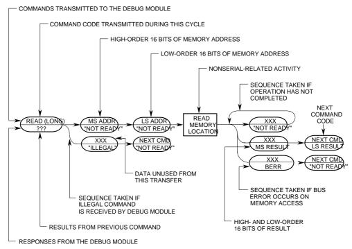
Figure 5-16, Command Sequence Diagram
