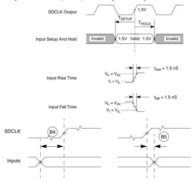
Figure 23-2. General Input Timing Requirements
