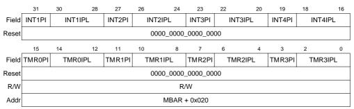
Figure 7-2. Interrupt Control Register 1 (ICR1)
