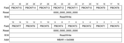
Figure 17-2. Port B Control Register (PBCNT)
