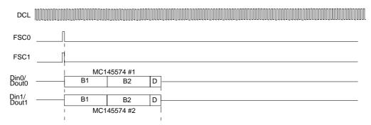
Figure 13-42. Standard IDL2 8-Bit mode
