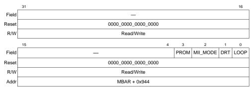
Figure 11-16. Receive Control Register (RCR)
