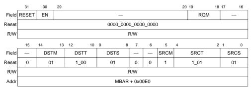
Figure 10-1. DMA Mode Register (DMR)
