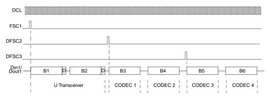
Figure 13-40. Standard IDL2 10-bit mode.
