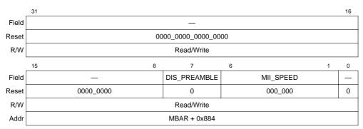
Figure 11-11. MII Speed Control Register (MSCR)
