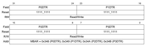
Figure 13-18. D Transmit Data Registers P0DTR-P3DTR
