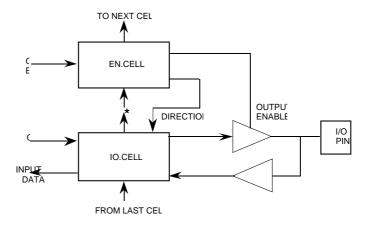
NOTE: More than one IO.Cell could be serially connected and controlled by a single En.Cell.
