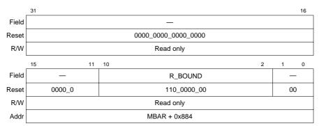
Figure 11-12. FIFO Receive Bound Register (FRBR)
