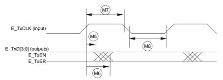
Figure 23-12. MII Transmit Signal Timing Diagram
