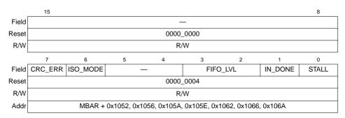
Figure 12-17. USB Endpoint 1-7 Control Register (EPnCTL)
