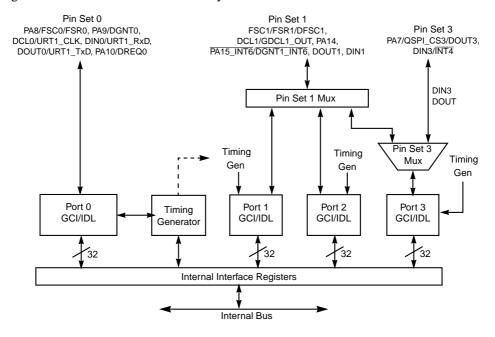
Figure 13-1. PLIC System Diagram
