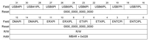
Figure 7-4. Interrupt Control Register 3 (ICR3)
