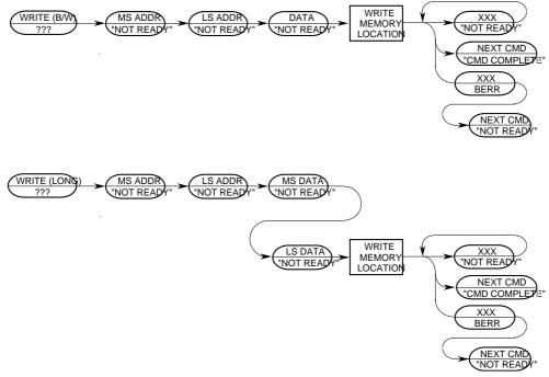
Figure 5-24. WRITE Command Sequence
