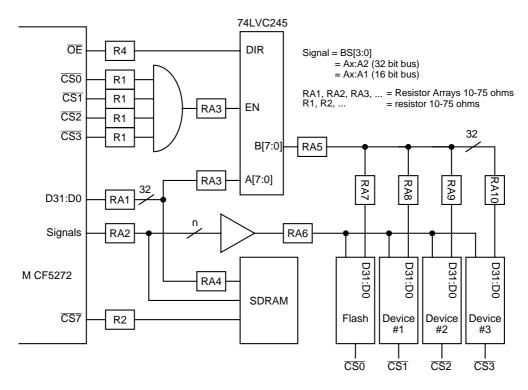
Figure B-1. Buffering and Termination
