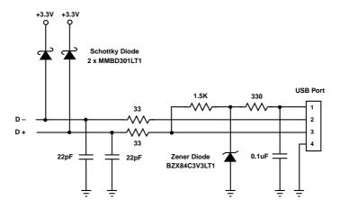
Figure 12-25. USB Protection Circuit
