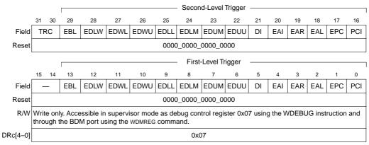
Figure 5-11. Trigger Definition Register (TDR)
