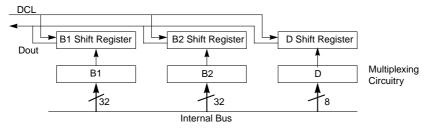
Figure 13-4. GCI/IDL Transmit Data Flow
