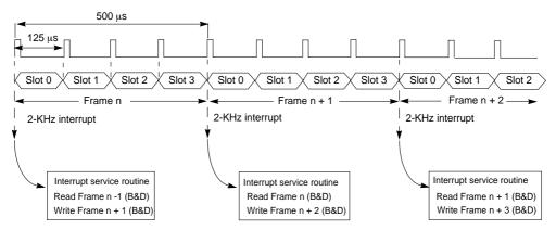
Figure 13-10. Periodic Frame Interrupt
