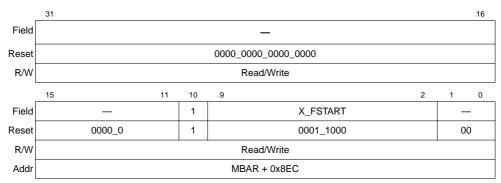
Figure 11-15. FIFO Transmit Start Register (TFSR)
