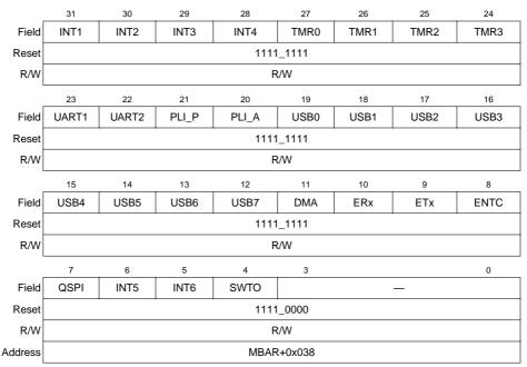
Figure 7-8. Programmable Interrupt Wakeup Register (PIWR)
