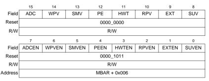
Figure 6-4. System Protection Register (SPR)
