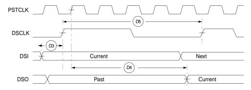
Figure 23-8. BDM Serial Port AC Timing
