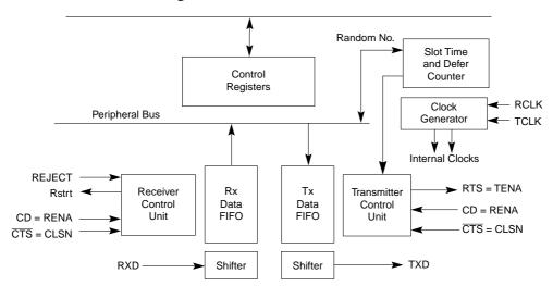
Figure 11-1. Ethernet Block Diagram
