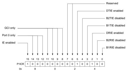
Figure 13-36. Port 1 Interrupt Configuration Register (P1ICR)
