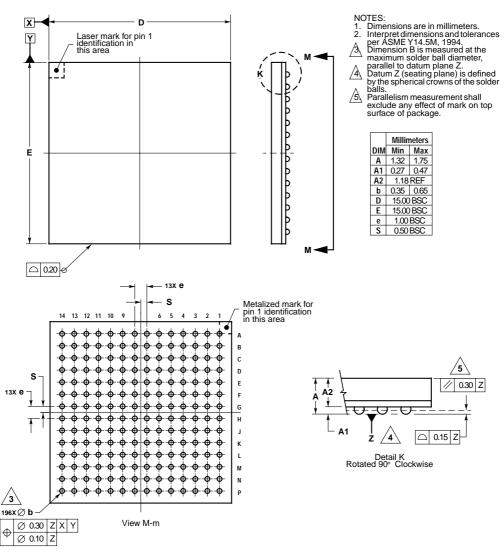
Figure 22-2. 196 MAPBGA Package Dimensions (Case No. 1128A-01)
