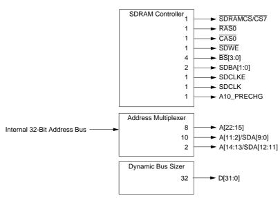
Figure 9-1. SDRAM Controller Signals
