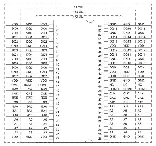
Figure 9-2. 54-Pin TSOP SDRAM Pin Definition
