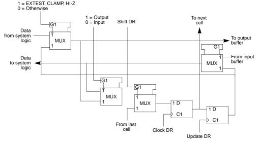
Figure 21-6. Bidirectional Cell (IO.Cell) (BC-6)
