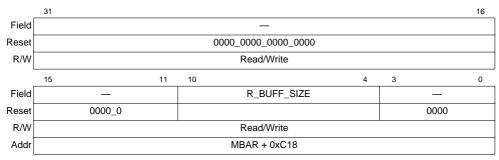
Figure 11-25. Receive Buffer Size (EMRBR)
