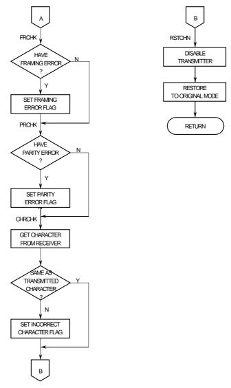
Figure 16-31. UART Mode Programming Flowchart (Sheet 3 of 5)
