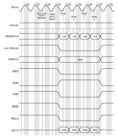
Figure 9-12. SDRAM Burst Write, 32-Bit Port, Page Hit, Access = 3-1-1-1
