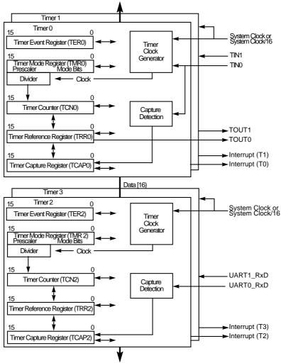
Figure 15-1. Timer Block Diagram
