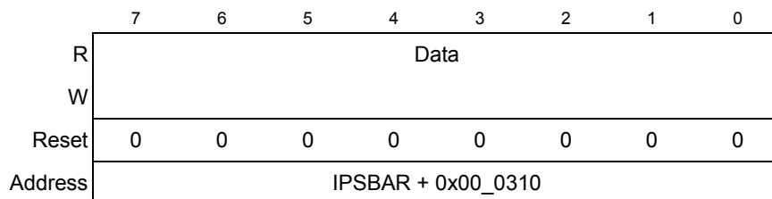
Figure 27-13. I 2 C Data I/O Register (I2DR)
