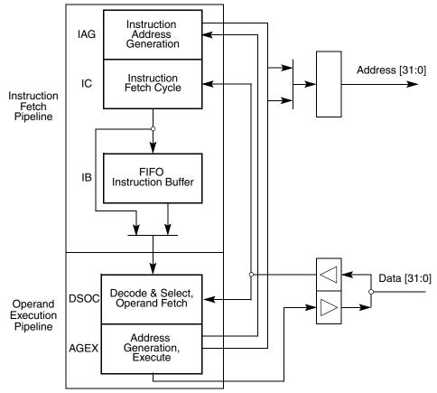
Figure 3-1. V2 ColdFire Core Pipelines
