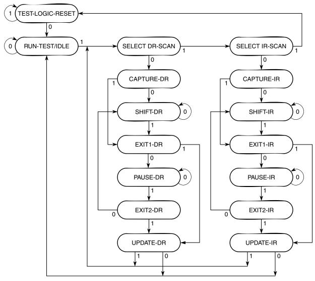
Figure 27-4. TAP Controller State Machine Flow
