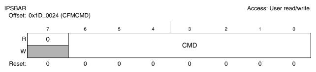
Figure 15-12. CFM Command Buffer and Register (CFMCMD)
