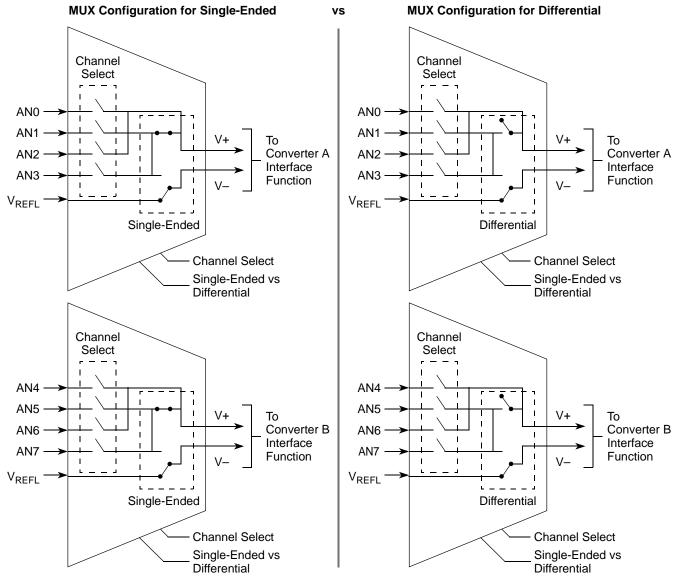
Figure 23-20. Input Select Mux
