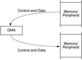
Figure 14-2. Dual-Address Transfer
