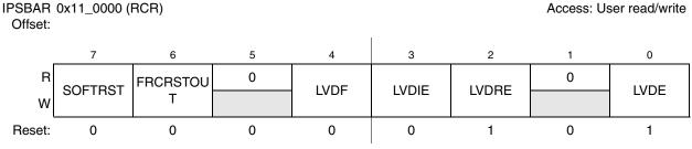
Figure 9-2. Reset Control Register (RCR)
