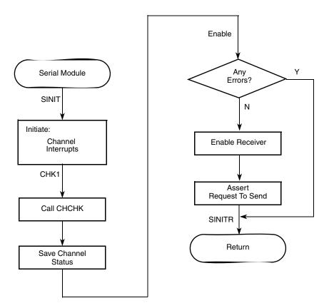
Figure 21-25. UART Mode Programming Flowchart (Sheet 1 of 5)
