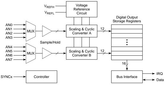
Figure 23-1. Dual ADC Block Diagram
