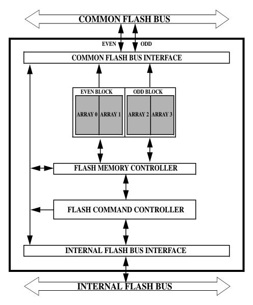
Figure 15-1. CFM Block Diagram
