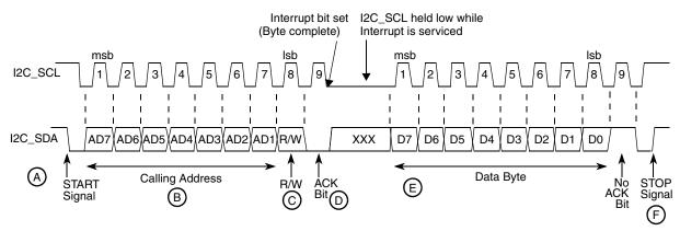
Figure 22-7. I<sup>2</sup>C Standard Communication Protocol
