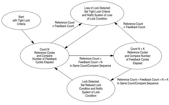
Figure 6-6. Lock Detect Sequence
