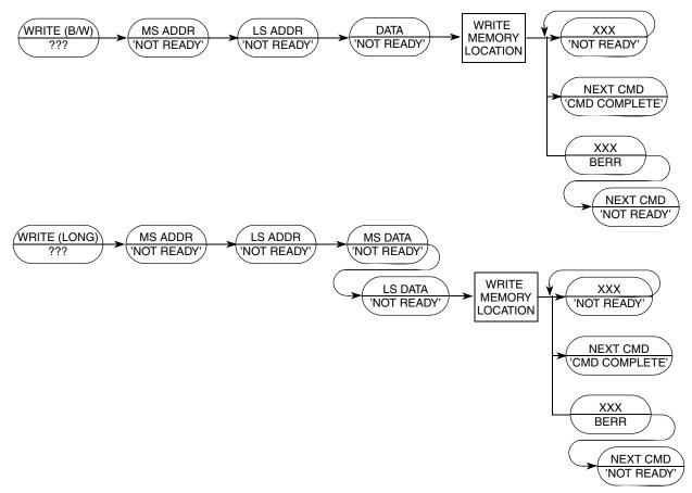
Figure 26-25. WRITE Command Sequence
