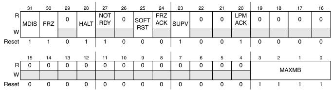
Figure 25-4. FlexCAN Configuration Register (CANMCR)
