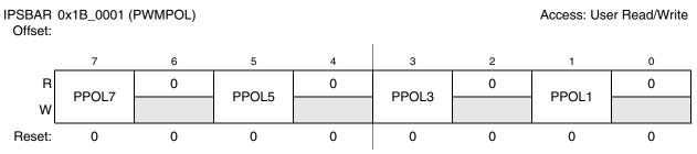
Figure 24-3. PWM Polarity Register (PWMPOL)
