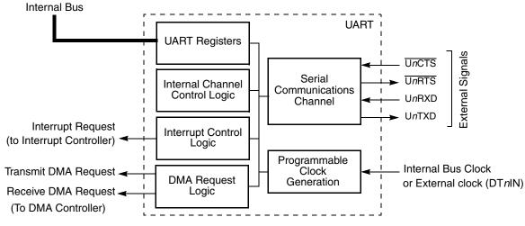
Figure 21-1. UART Block Diagram
