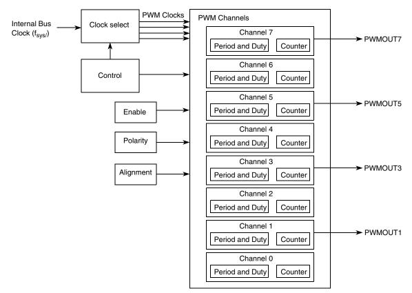
Figure 24-1. PWM Block Diagram
