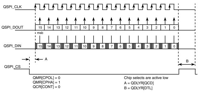
Figure 20-3 shows an example of a QSPI clocking and data transfer.
