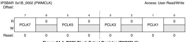
Figure 24-4. PWM Clock Select Register (PWMCLK)
