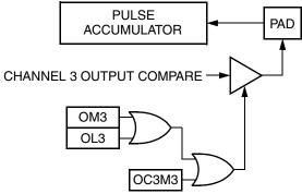
Figure 18-22. Channel 3 Output Compare/Pulse Accumulator Logic
