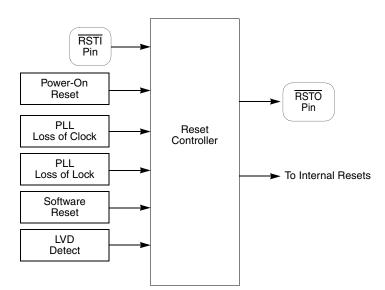
Figure 9-1. Reset Controller Block Diagram
