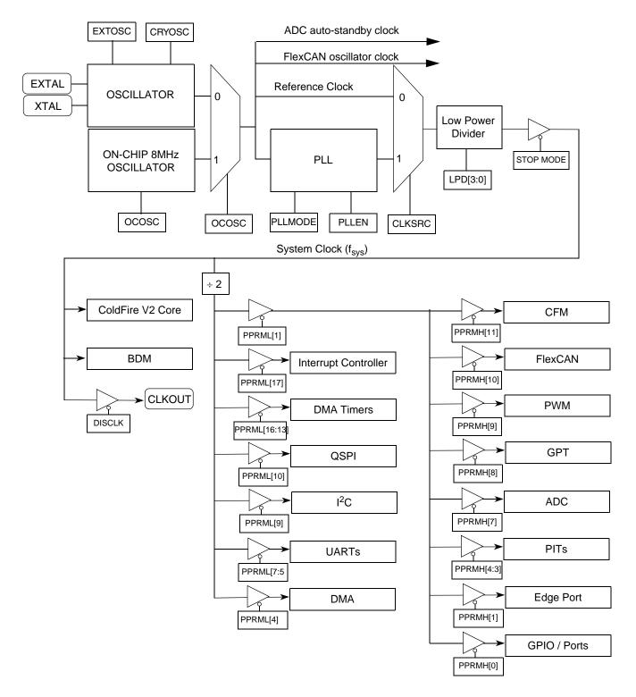
Figure 6-1. Clock Module Block Diagram
