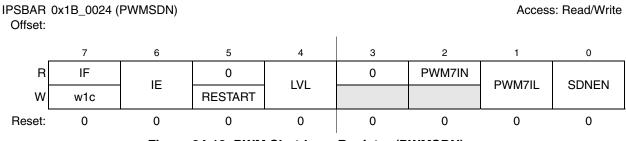
Figure 24-13. PWM Shutdown Register (PWMSDN)
