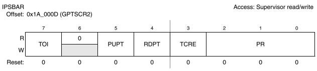
Figure 18-13. GPT System Control Register 2 (GPTSCR2)
