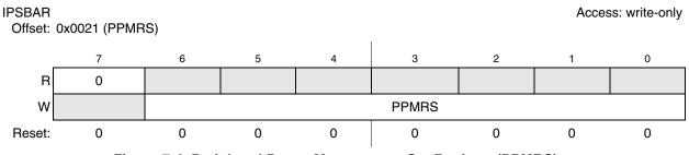
Figure 7-4. Peripheral Power Management Set Register (PPMRS)
