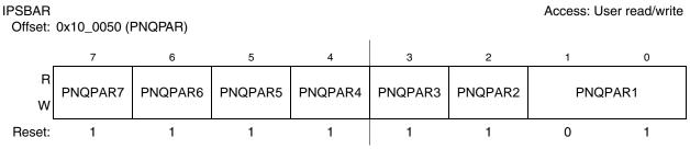
Figure 11-27. Port NQ Pin Assignment Register (PNQPAR)
