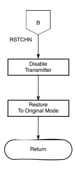
Figure 21-25. UART Mode Programming Flowchart (Sheet 3 of 5)
