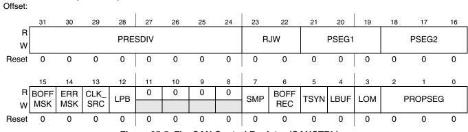
Figure 25-5. FlexCAN Control Register (CANCTRL)
