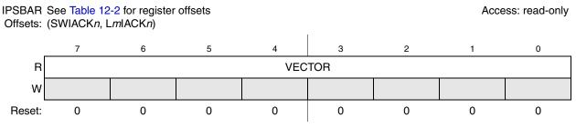
Figure 12-10. Software and Level m IACK Registers (SWIACKn, LmIACKn)
