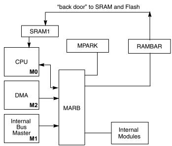
Figure 10-6. Arbiter Module Functions
