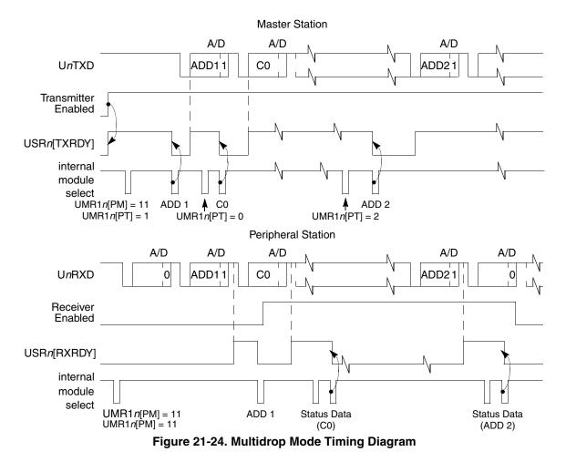
A character sent from the master station consists of a start bit, a programmed number of data bits, an address/data (A/D) bit flag, and a programmed number of stop bits. A/D equals 1 indicates an address character; A/D equals 0 indicates a data character. The polarity of A/D is selected through UMR1n[PT]. UMR1n should be programmed before enabling the transmitter and loading the corresponding data bits into the transmit buffer.
