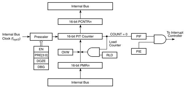
Figure 17-1. PIT Block Diagram
