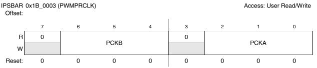
Figure 24-5. PWM Prescale Clock Select Register (PWMPRCLK)
