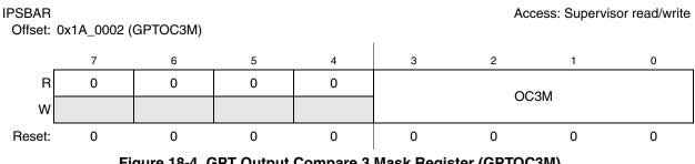
Figure 18-4. GPT Output Compare 3 Mask Register (GPTOC3M)
