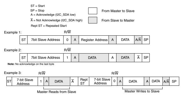
Figure 22-11. Data Transfer, Combined Format
