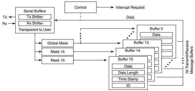
Figure 25-2. FlexCAN Message Buffer Architecture
