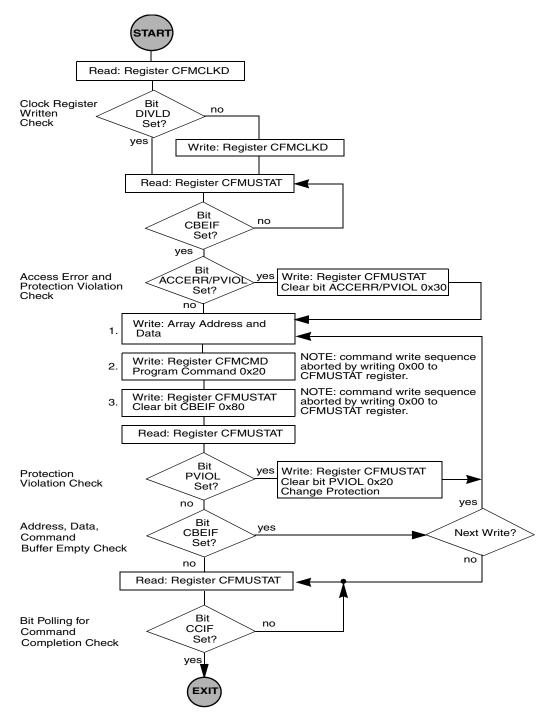
Figure 15-16. Example Program Command Flow
