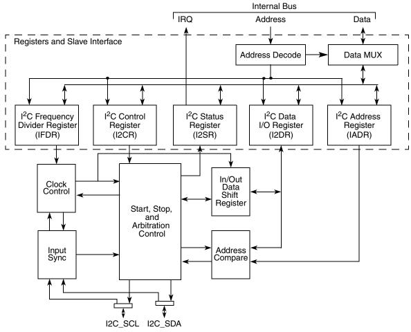
Figure 22-1. I<sup>2</sup>C Module Block Diagram
