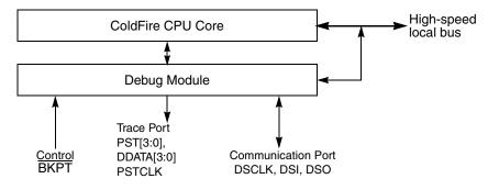
Figure 26-1. Processor/Debug Module Interface
