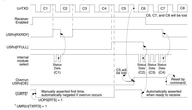
Figure 21-20 shows receiver functional timing.
