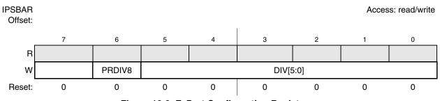
Figure 16-3. EzPort Configuration Register
