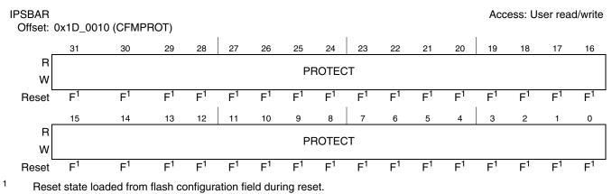
Figure 15-7. CFM Protection Register (CFMPROT)
