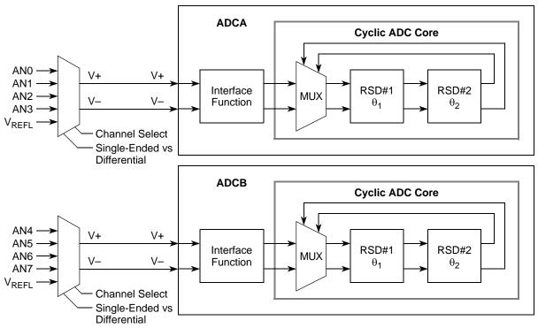
Figure 23-21. Cyclic ADC – Top Level Block Diagram
