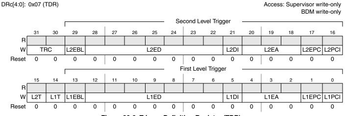
Figure 26-6. Trigger Definition Register (TDR)
