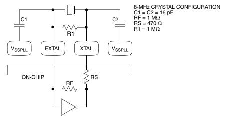
Figure 6-5. Crystal Oscillator Example
