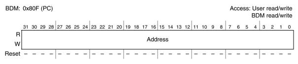
Figure 3-6. Program Counter Register (PC)
