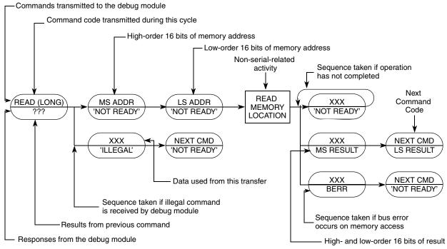
Figure 26-17. Command Sequence Diagram
