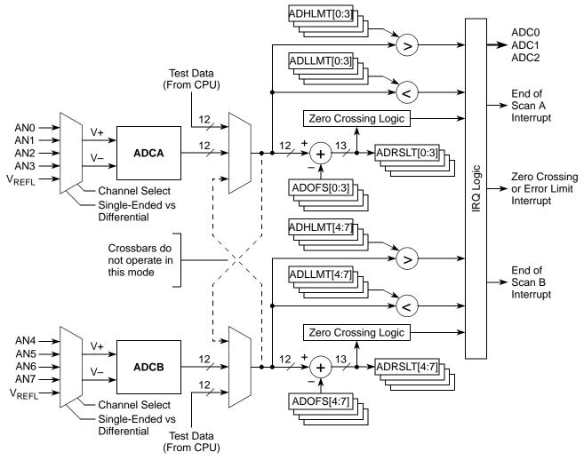
Figure 23-19. Parallel Mode Operation of the ADC
