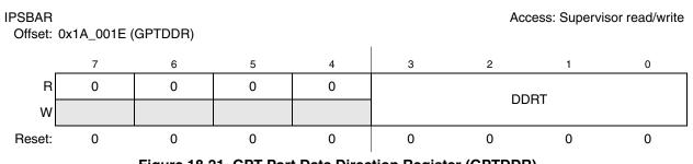
Figure 18-21. GPT Port Data Direction Register (GPTDDR)
