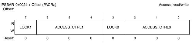
Figure 10-9. Peripheral Access Control Register (PACRn)
