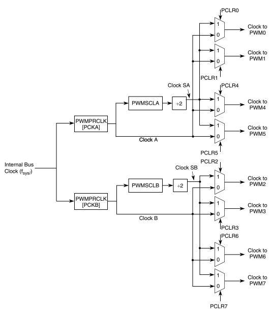
Figure 24-14. PWM Clock Select Block Diagram
