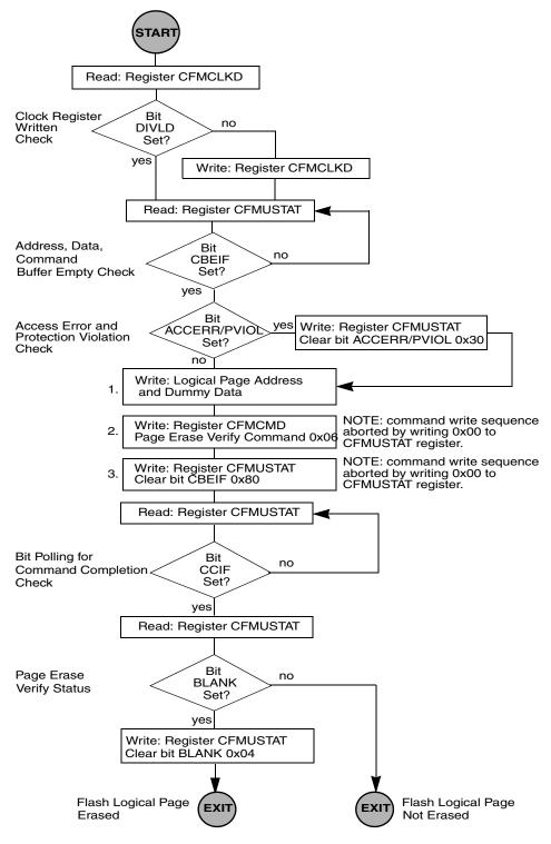
Figure 15-15. Example Page Erase Verify Command Flow
