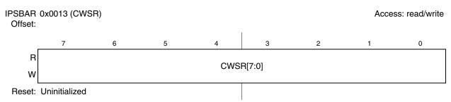
Figure 10-5. Core Watchdog Service Register (CWSR)
