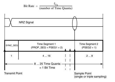
Figure 25-15. Segments within the Bit Time
