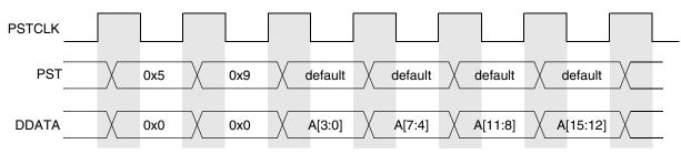
Figure 26-2. Example JMP Instruction Output on PST/DDATA
