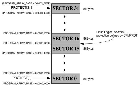
Figure 15-8. CFMPROT Protection Diagram
