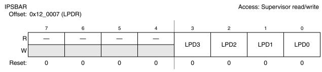
Figure 6-4. Low-Power Divider Register (LPDR)
