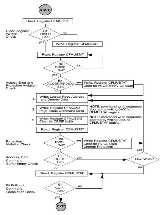
Figure 15-17. Example Page Erase Command Flow
