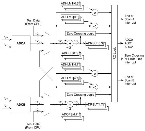
Figure 23-23. Result Register Data Manipulation
