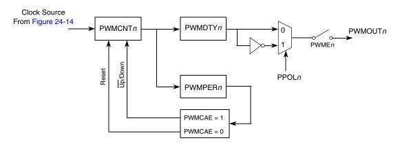
Figure 24-15. PWM Timer Channel Block Diagram
