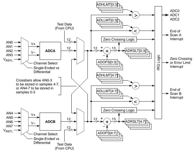
Figure 23-18. Sequential Mode Operation of the ADC
