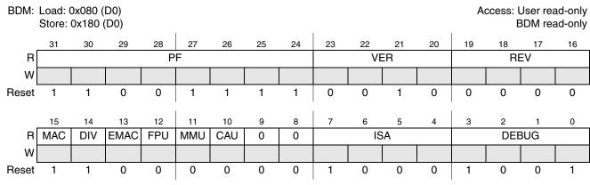
Figure 3-11. D0 Hardware Configuration Info
