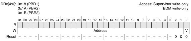
Figure 26-8. PC Breakpoint Register n (PBRn)
