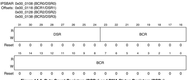
Figure 14-6. Byte Count Registers (BCRn) and DMA Status Registers (DSRn)
