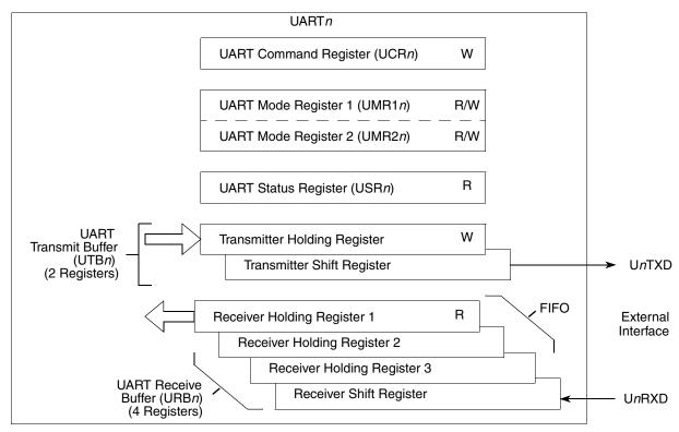
Figure 21-18. Transmitter and Receiver Functional Diagram
