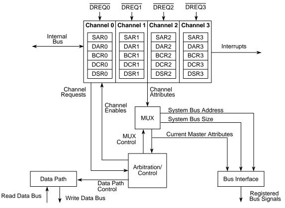
Figure 14-1. DMA Signal Diagram
