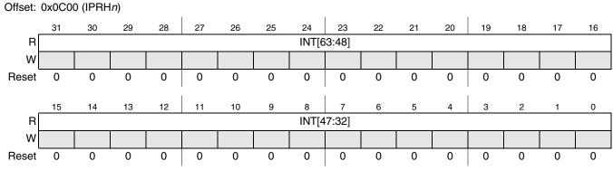
Figure 12-1. Interrupt Pending Register High (IPRHn)
