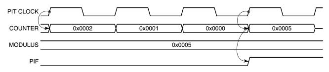
Figure 17-5. Counter Reloading from the Modulus Latch
