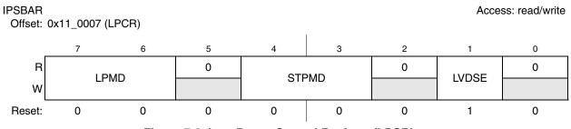
Figure 7-6. Low-Power Control Register (LPCR)
