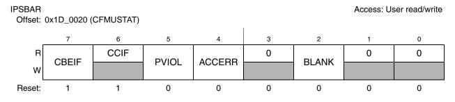
Figure 15-11. CFM User Status Register (CFMUSTAT)
