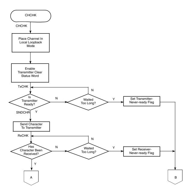
Figure 21-25. UART Mode Programming Flowchart (Sheet 2 of 5)
