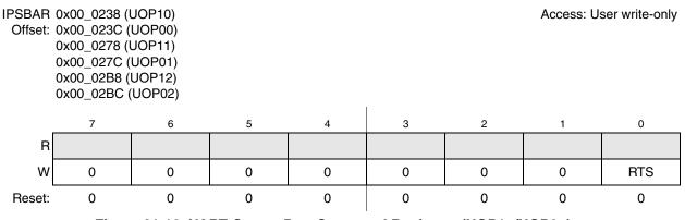
Figure 21-16. UART Output Port Command Registers (UOP1n/UOP0n)
