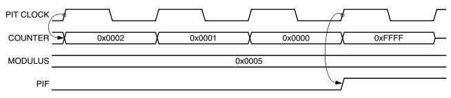
Figure 17-6. Counter in Free-Running Mode
