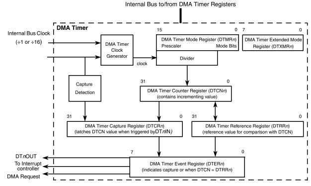
Figure 19-1 is a block diagram of one of the four identical timer modules.
