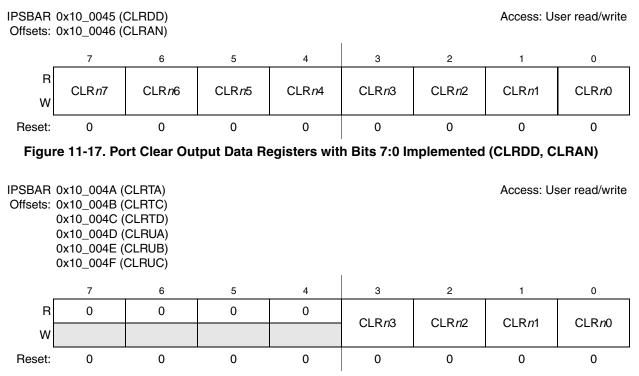
Figure 11-18. Port Clear Output Data Registers with Bits 3:0 Implemented (CLRTA, CLRTC, CLRTD, CLRUA, CLRUB, CLRUB, CLRUC)
