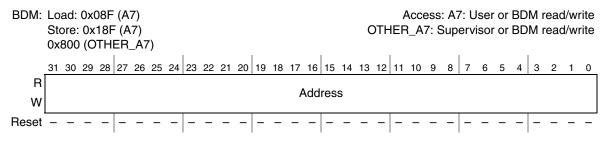
Figure 3-4. Stack Pointer Registers (A7 and OTHER\_A7)
