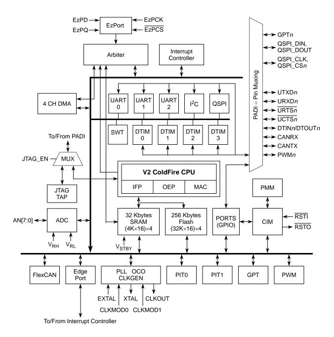
Figure 1-1. MCF5213 Block Diagram
