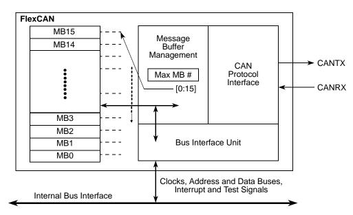
Figure 25-1. FlexCAN Block Diagram
