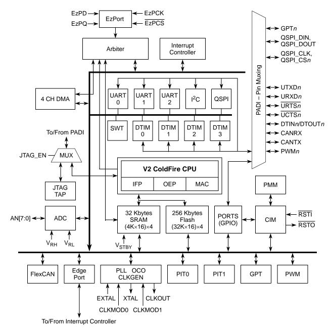
Figure 2-1. Block Diagram with Signal Interfaces
