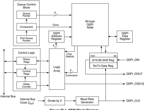
Figure 20-1. QSPI Block Diagram
