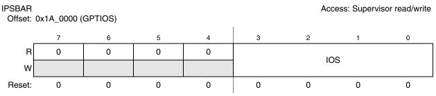
Figure 18-2. GPT Input Capture/Output Compare Select Register (GPTIOS)
