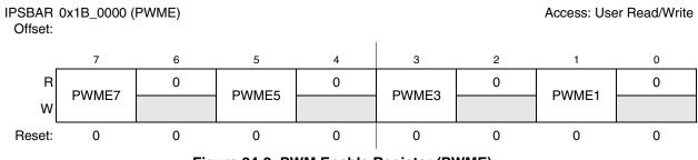
Figure 24-2. PWM Enable Register (PWME)
