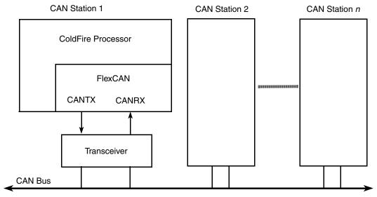
Figure 25-3. Typical CAN System
