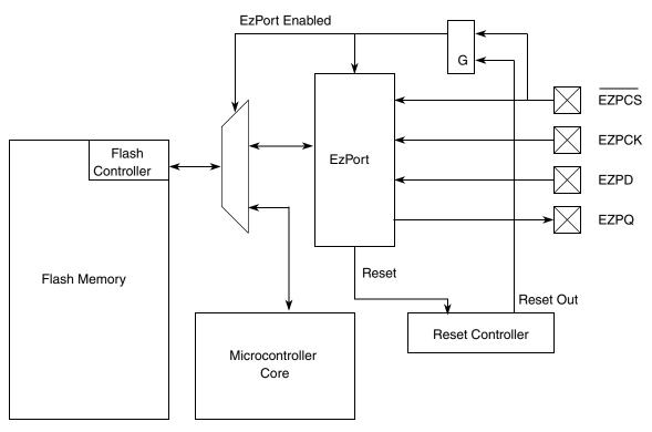
Figure 16-1. EzPort Block Diagram
