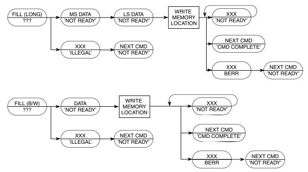
Figure 26-29. FILL Command Sequence
