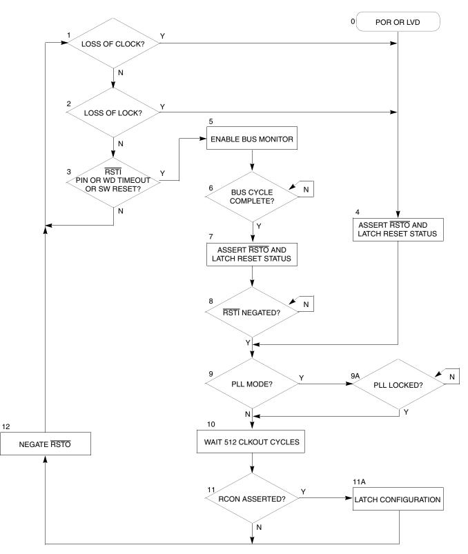
Figure 9-4. Reset Control Flow
