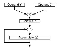
Figure 4-1. Multiply-Accumulate Functionality Diagram
