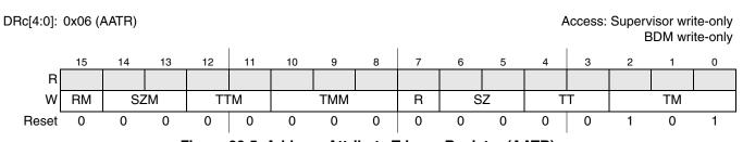
Figure 26-5. Address Attribute Trigger Register (AATR)
