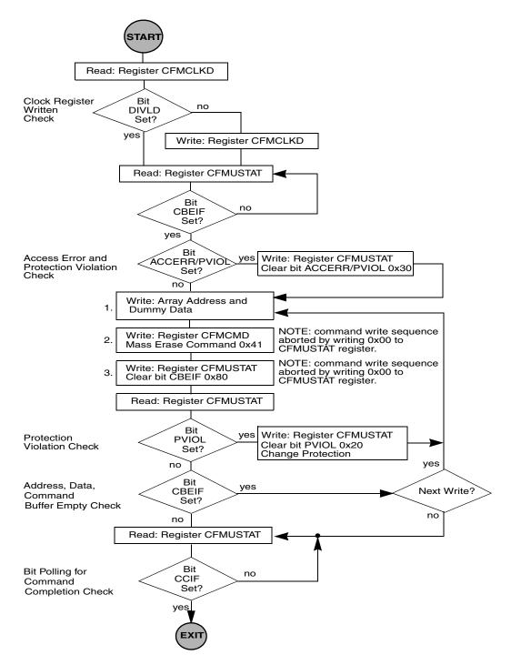
Figure 15-18. Example Mass Erase Command Flow
