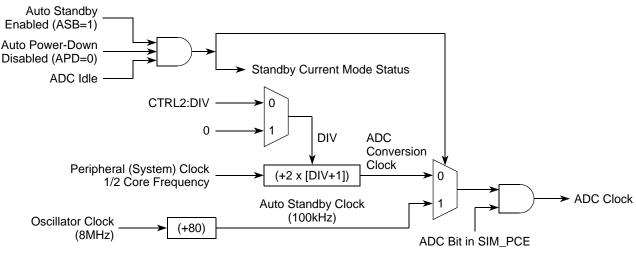
Figure 23-25. ADC Clock Generation
