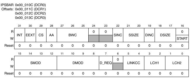
Figure 14-8. DMA Control Registers (DCRn)
