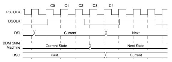
Figure 26-13. Maximum BDM Serial Interface Timing
