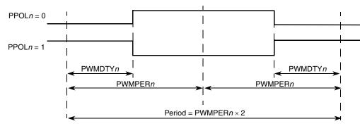
Figure 24-18. PWM Center-Aligned Output Waveform
