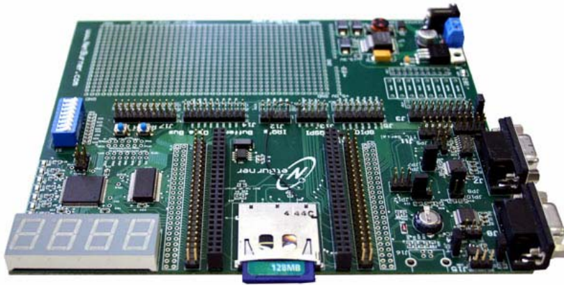
NetBurner Development Board showing SD/MMC card interface (network module has been removed).
