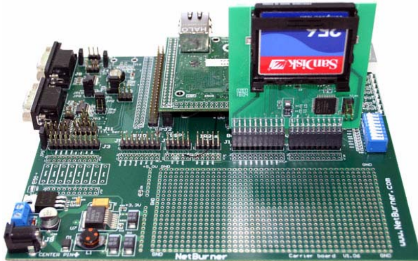
NetBurner Development Board showing Compact Flash card interface
