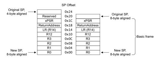
Figure B1-3 Alignment options when stacking the basic frame
