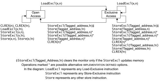
Any LoadExcl operation updates the tagged address to the most significant bits of the address x used for the operation. See text for more information about tagging.
