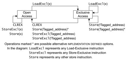
Any LoadExcl operation updates the tagged address to the most significant bits of the address x used for the operation. See text for more information about tagging.
