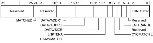
‡ DWT\_FUNCTION0 only, bit [7] is Reserved in all other DWT\_FUNCTIONn registers.
